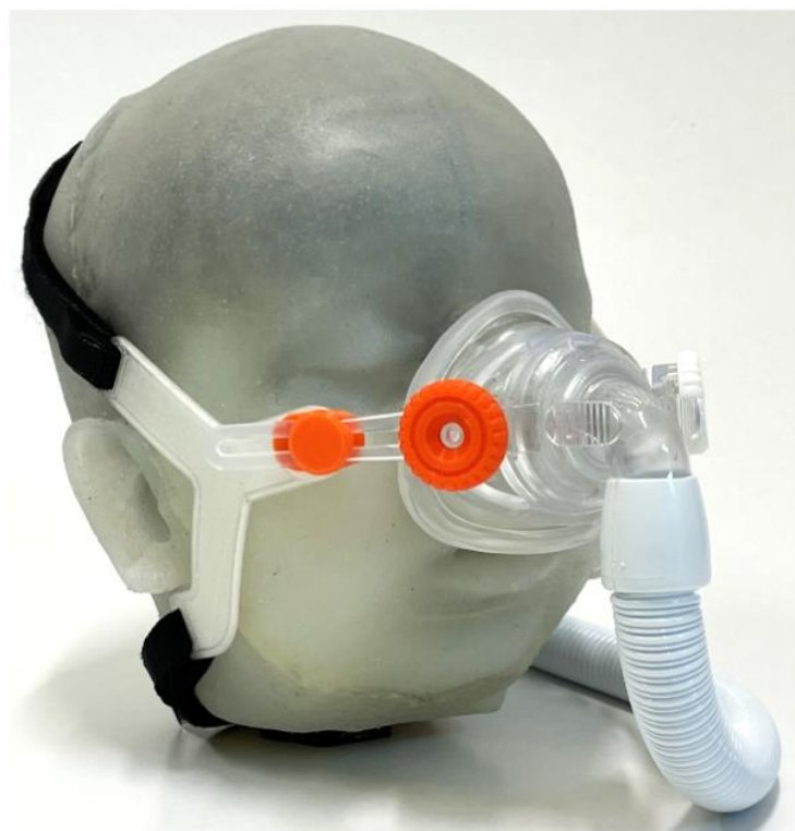
Figure 1. Prototypical Custom-Made Mask and Headgear on a Paediatric Dummy Head.
