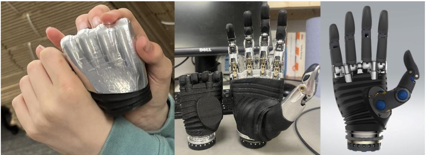
L to R: a hand chassis prototype from early PPI work, chassis relative to a bionic small, current Rebel hand design.
